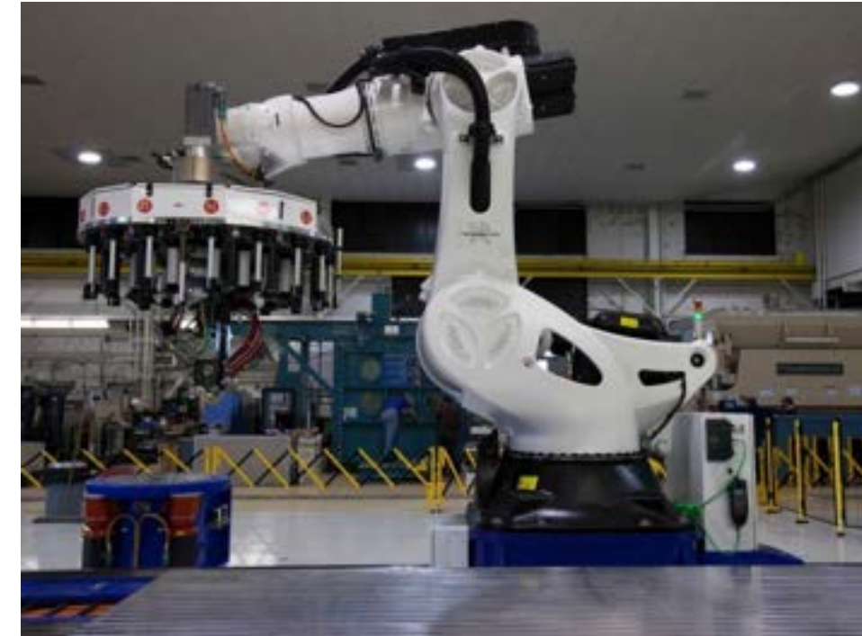
ISAAC (Electro Impact) AFP Machine, NASA Langley
