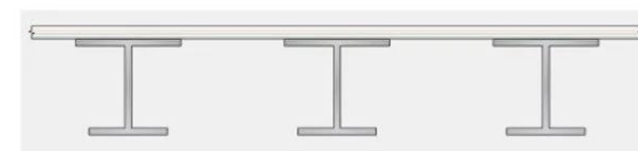
Both FEMs are “I” stiffened panels
