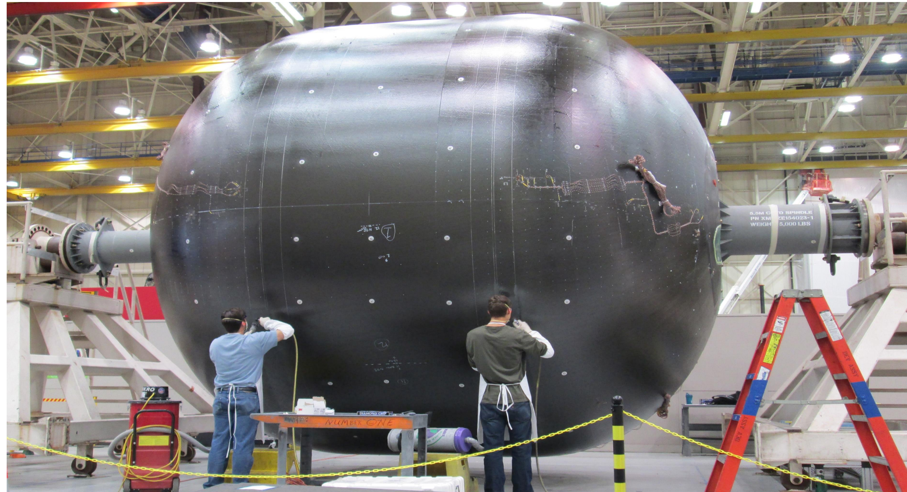
NASA/Boeing Composite Cryotank Demonstration 5.5 m (2015)
