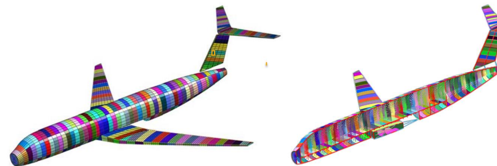
Figure 11. Global Structural Finite Element Model
