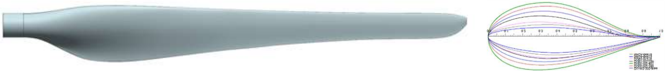
Fig. 3 Optimum planform of 30 kW wind blade
